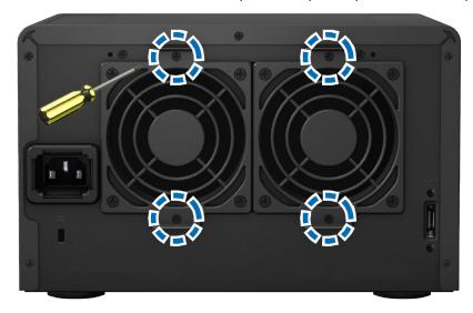
**4** Remove the malfunctioning fans by disconnecting the fan cable from the connectors.
