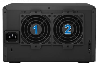
3 Remove the screws that secure the fan panels and pull the panels from the expansion unit.
