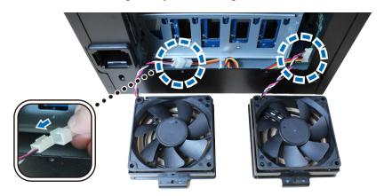
5 Connect the cables of the new fans to the connectors and tighten the screws removed in step 3.
